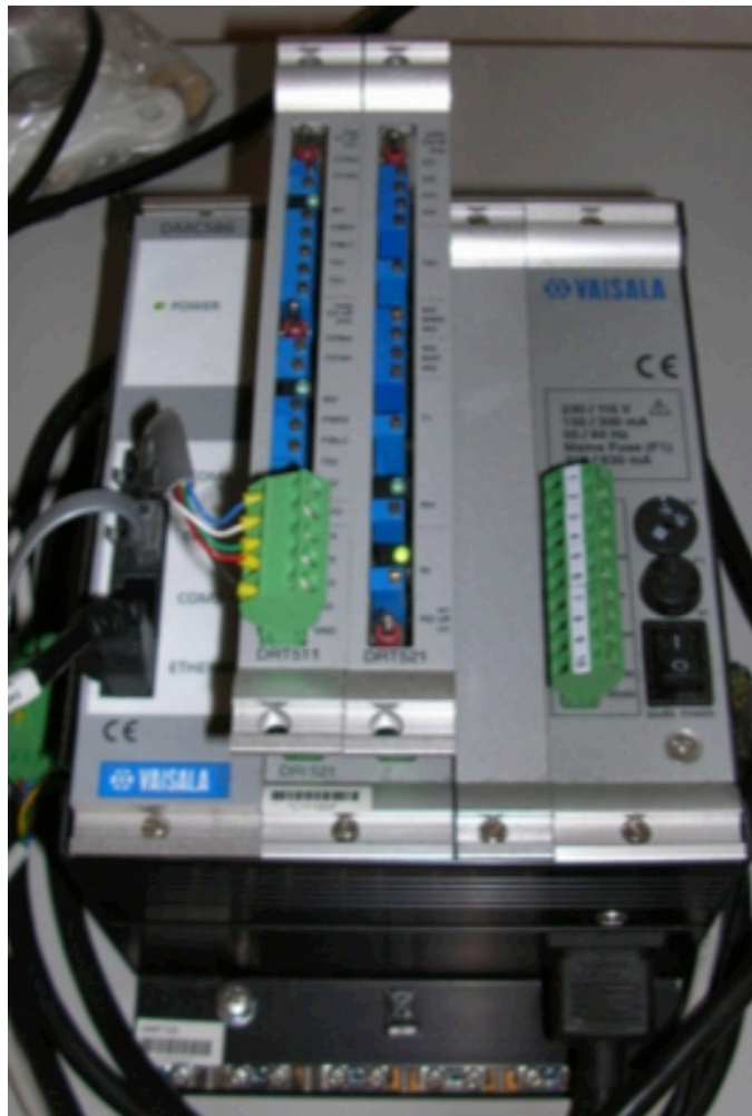
Figure 3-1: Vaisala RPU Used for Limited SunGuide Software Functional Testing
